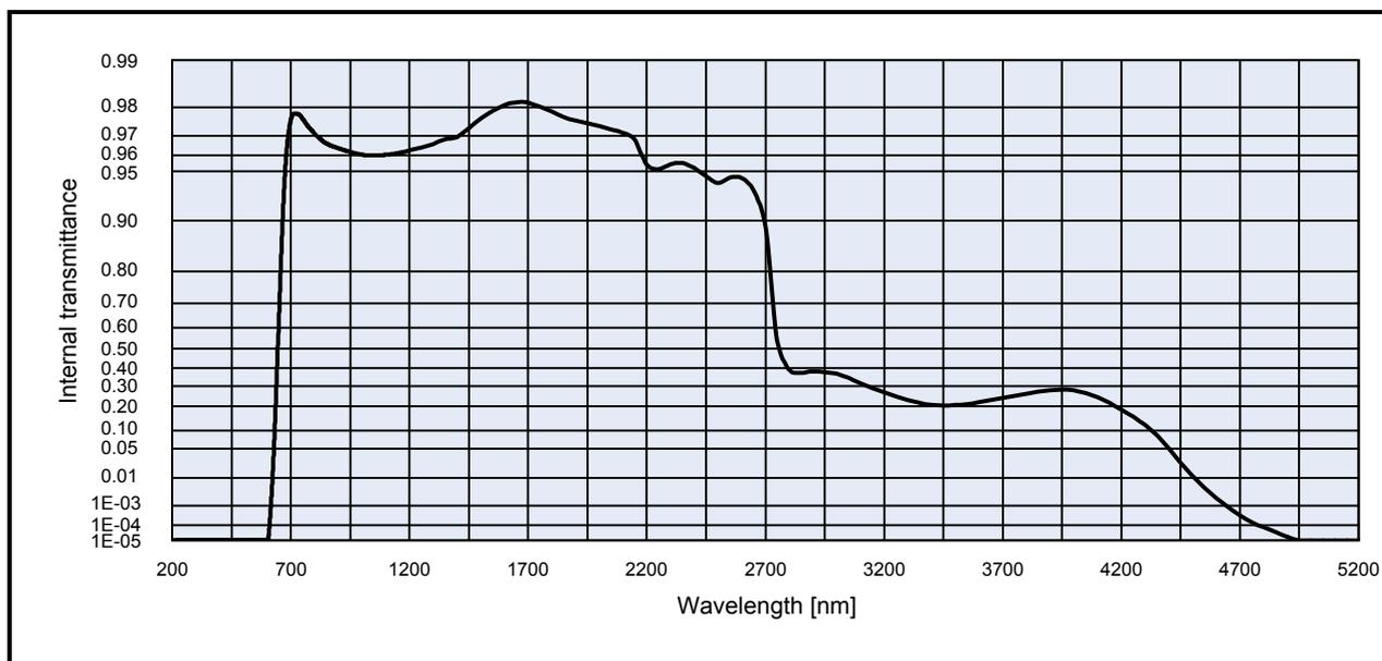
**Internal transmittance  $\tau_i$  at reference thickness  $d$  [mm] = 3**
